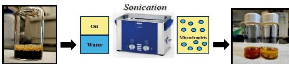
Figure 1. Schematic and visual representation of how lignin is transformed into other products through Emulsive microdroplets generated through sonication
